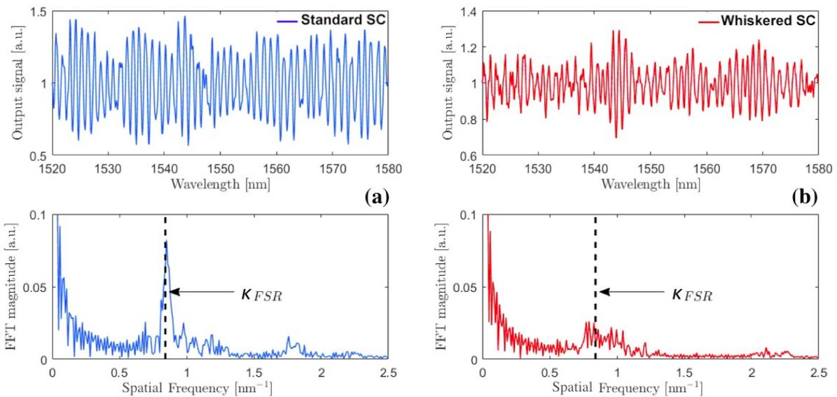
Figure 2. (top - a and b ) Fabry-Perot (FP) interference evaluated by injecting a tunable IR laser within both the structures showed in Fig.1(a) and (b). We identified as the FP facets the input focal line of the SCs and the ending facets of the waveguide of the array. (bottom - a and b) FFT performed on the experimental spectra. The dashed line represents the spatial frequency predicted by FP theory.
