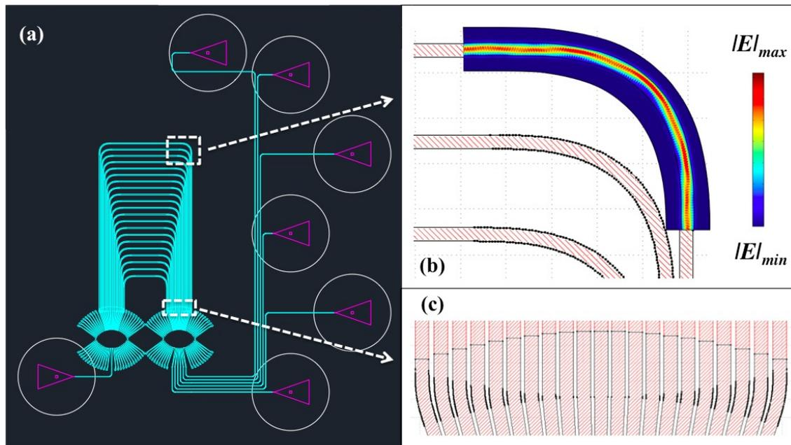
Figure 3. (a) AWG layout: in cyan the silicon waveguides, in magenta the grating couples. (b) FEM simulation of the electric field profile propagating through the Bezier bending geometry realized for minimizing the footprint. (c) Bezier bendings adopted instead of circular arcs at the SC/array junction.
