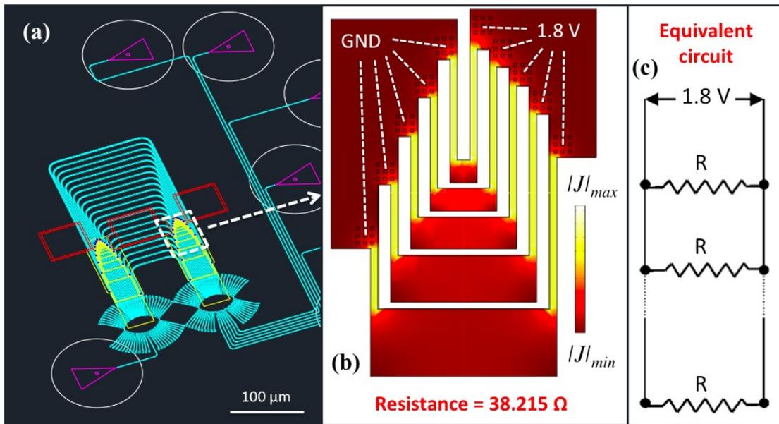
Figure 4. (a) AWG layout with heating elements: in cyan the silicon waveguides, in magenta the grating couplers, in yellow the Ti/TiN heaters, in blue the copper vias, in red the electric pads (b) FEM simulation of current density through the heater when the bias is switched on. (c) Equivalent circuit where it can be seen that the strips have been dimensioned to obtain the same resistance value for each arm.
