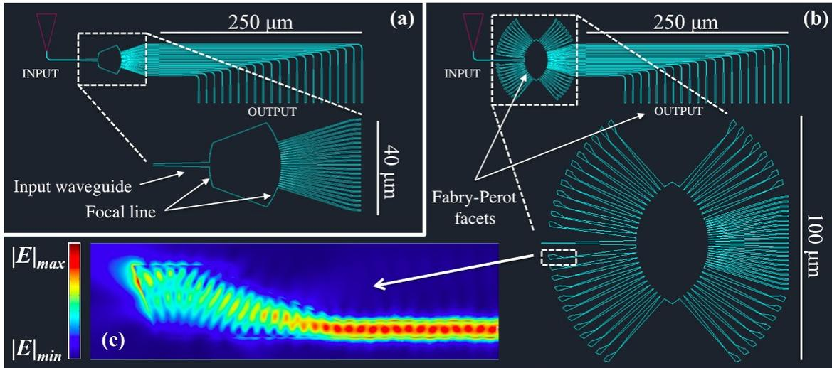
Figure 1. (a) Standard SC with 1 input waveguide and 21 output waveguides. (b) Whiskered SC with 1 input waveguide and 21 output waveguides. (c) FEM simulation of the electric field profile propagating through the "reflection killer" geometry.
